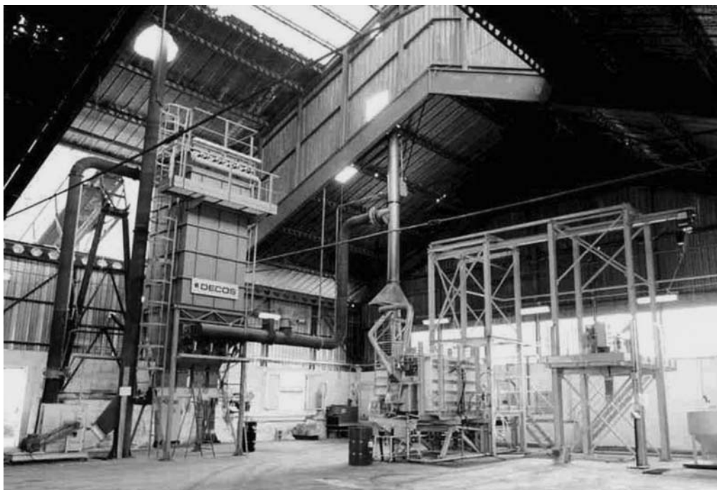
Figure 11 Photo of the pilot plant for production of glass-ceramic tiles from industrial wastes, situated in Iglesias, Italy [177]. (Photo courtesy Prof. M. Pelino, University of L'Aquila, Italy).
